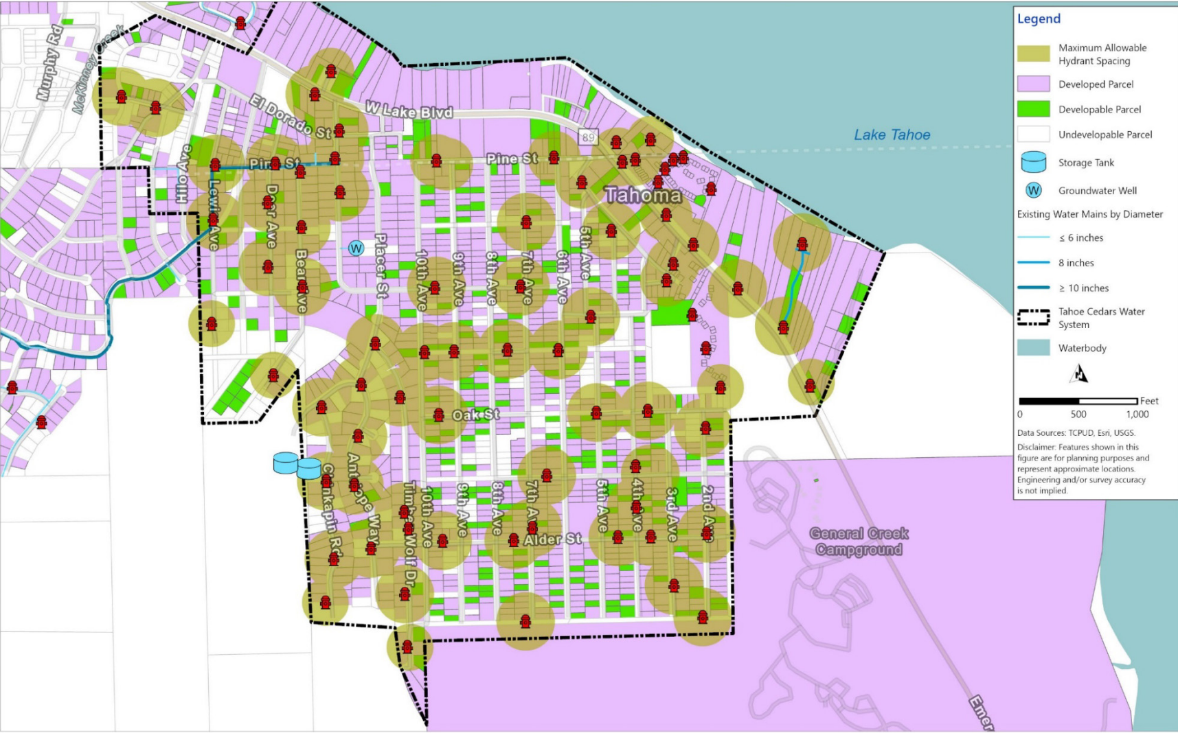
Figure 6 Tahoe Cedars Fire Hydrant Spacing - Alternative 1
