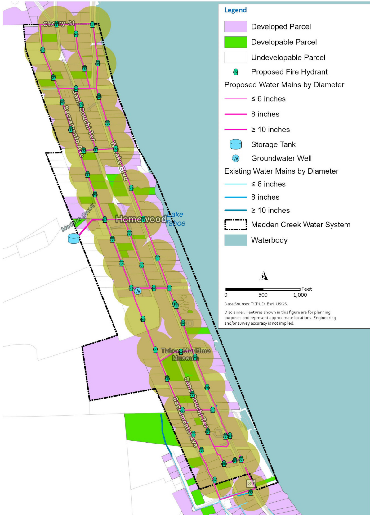
Figure 9 Madden Creek Fire Hydrant Spacing - Alternative 2
